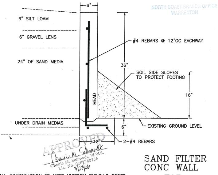
ALL CONSTRUCTION TO MEET UNIFORM BUILDING CODES CONCRETE TO BE 2500 PSI @ 28 DAYS REBAR TO BE GRADE 40 OR BETTER OWNER/CONTRACTOR TO OBTAIN BUILDING PERMIT IF REQUIRED FOR CONC BOX
