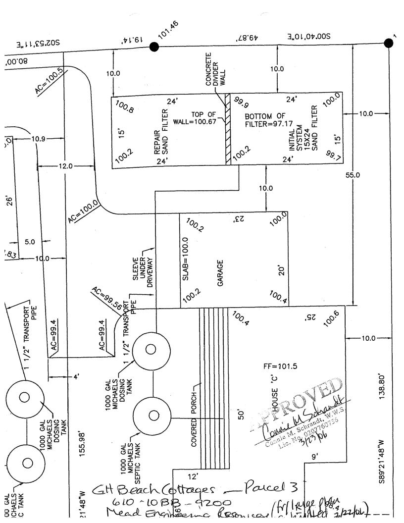
GH Beach Cottages 610 10BB 9200 Parcel 3 Mead Ergineering Resour M. MEAD @ AGLOVES PLYWOOD BOX IF NEEDED BY provide 1 1/4" FROM SEPTIC TANK OF DRAIN ROCK 1/4" MANIFOLD SOIL CAP SLOPE 90° SWEEP END CAP & PVC BOX PLAN BOTTOMLESS SAND FILTER SEE PLAN EXIST GROUND
