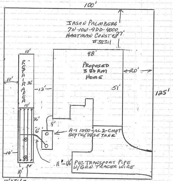
10'X36' BOTOMLESS SANDFILTER JASON MAX DEPTH 36" MIN. DEPTH 24"
